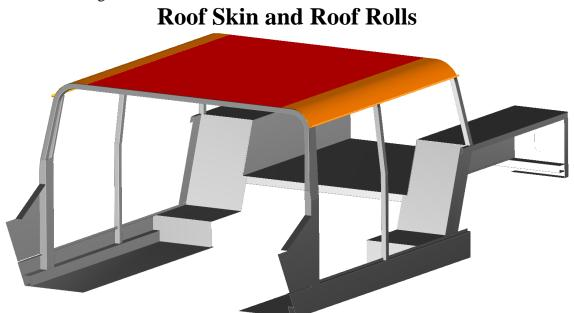
Center the roof skin (if applicable) after smoothing down any welds as necessary for fitment. Be sure to slide to the front for proper alignment of rear hatch alignment. Many times there is a little extra on the front that you can grind off after finish welding.
