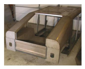
Position the tailgate side and bottom supports into place and grind for precise fitment. It is a good idea to work on a flat surface and align the flat sides down. You may even want to clamp down the tailgate to flatten the sides and then tack the side, bottom, and other side supports which can then hold the tailgate in a flat position. Once you have all the parts in place and everything is correct then you can then finish weld.
