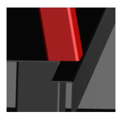
Use a long straightedge on each side to align the bed sides with the B-post and A-post. You can put some sheet metal in to space the A and B posts as necessary but may not matter as that is only 0.075" difference.
