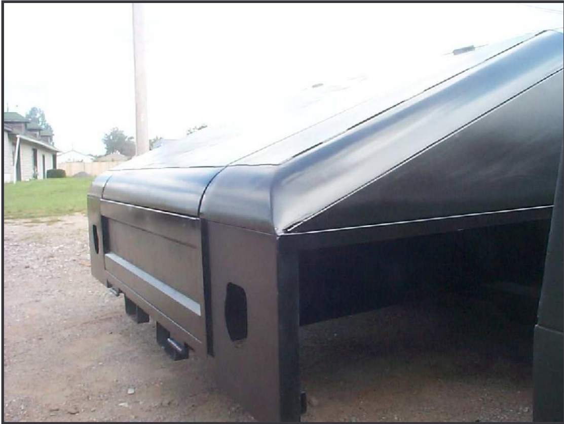
Fig 3-13: ...tailgate assembly attached to a slantback body...
