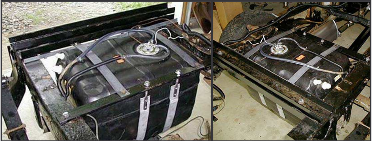
Fig 2-6: ...example of alternate gas tank installation...
