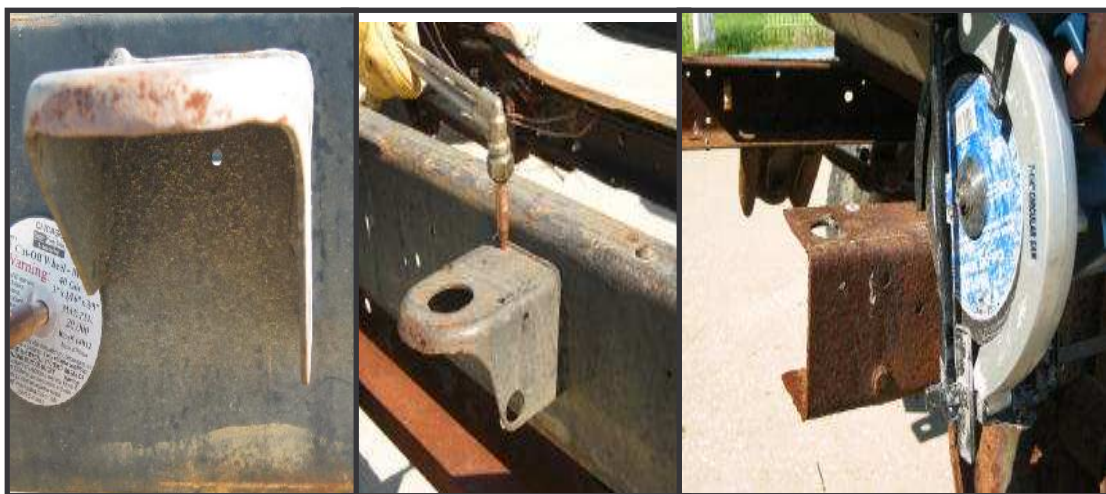
Fig 2-2: ...various methods available to remove old body mounts...
