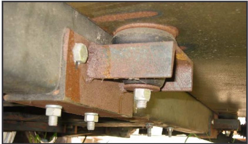
Fig 2-3: ...existing body mounts on late model Suburban...
